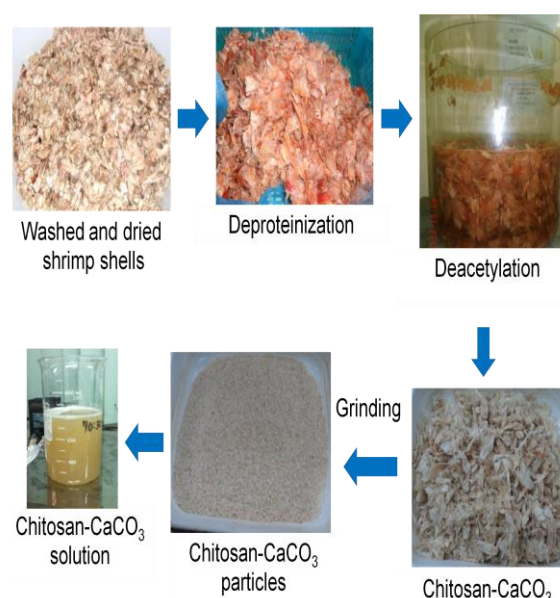
Figure 1. Process flow of Chitosan containing Calcium Carbonate extraction
