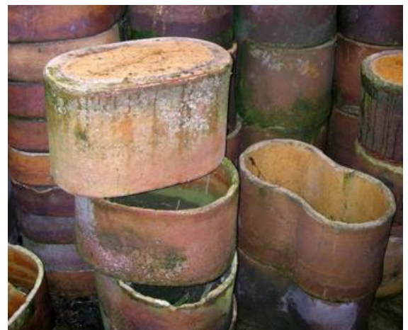
Figure 3: Saggarboxes, which use in Staffordshire ( http://www.carolventura.com/Jingdezhen.htm )
