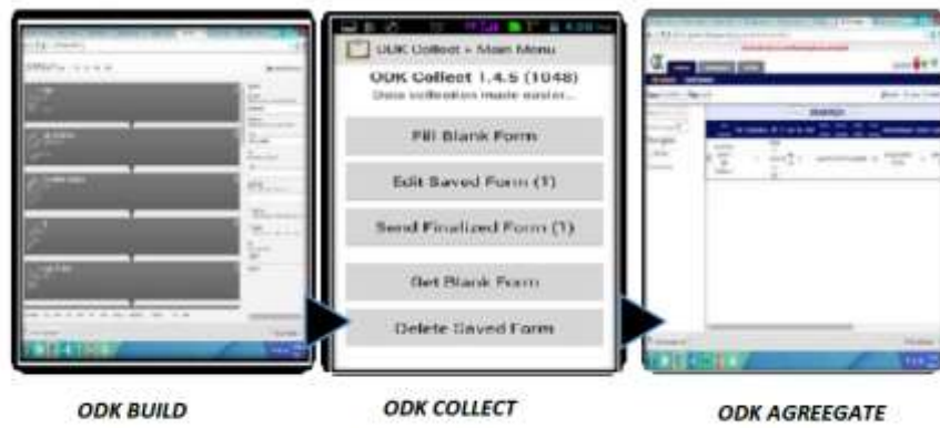
Figure.1: Process of preparing a survey form, collecting data and storage of data
